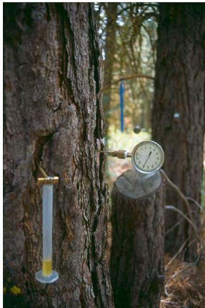
Figure 4. OEP and OEF measurements in a pole-size ponderosa pine (not in the study area), showing ~5 mL of resin and a pressure reading of approximately 1240 kPa. Note: in this study, OEP and OEF were NOT measured simultaneously.
